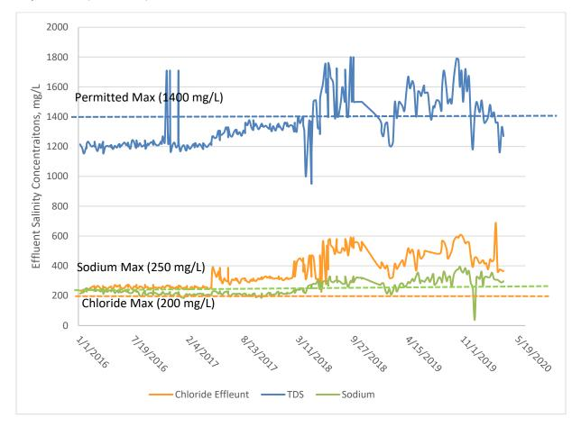
**Figure 13 Effluent Monthly Salinity Concentrations**
