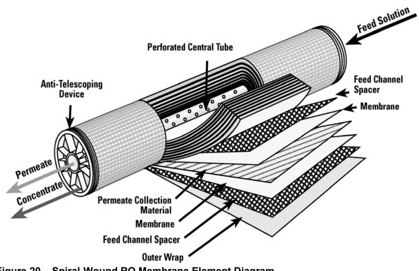
Figure 20 – Spiral-Wound RO Membrane Element Diagram
