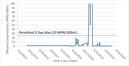
Figure 16 Five-Day Median Total Coliform Effluent Concentrations
