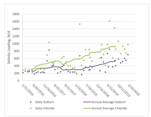
Figure 9 Influent Sodium and Chloride Loading
