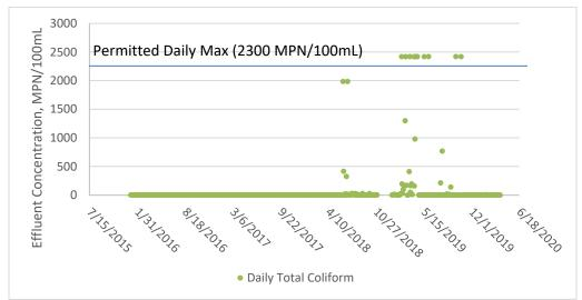
**Figure 15 Daily Total Coliform Effluent Concentrations**
