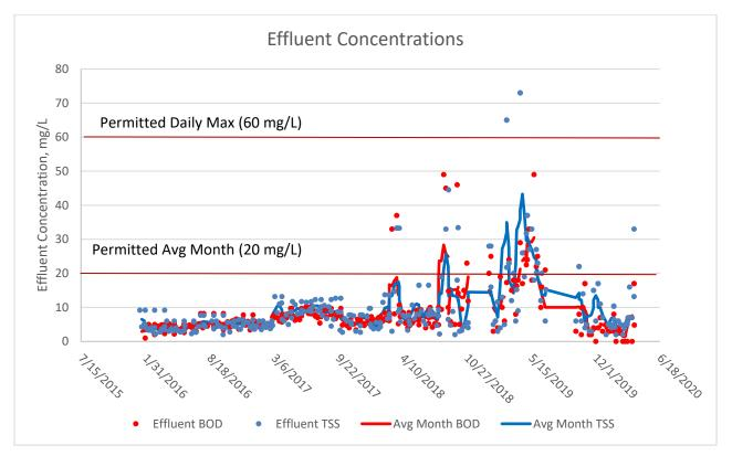
Figure 14 BOD and TSS Effluent Concentrations
