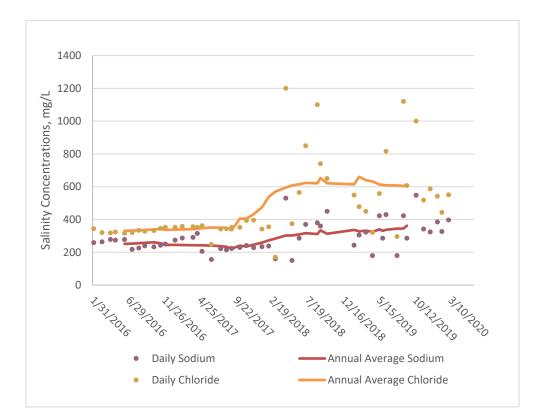
Figure 11 Influent Sodium and Chloride Concentrations
